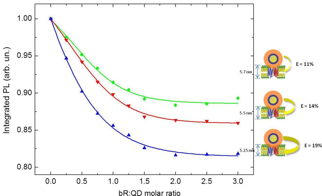
Figure 3. Experimental effects of pH-controlled variation of the thickness of the purple membrane (PM) on the efficiency of energy transfer from QDs to bR within self-assembled bR–QD hybrid materials.
