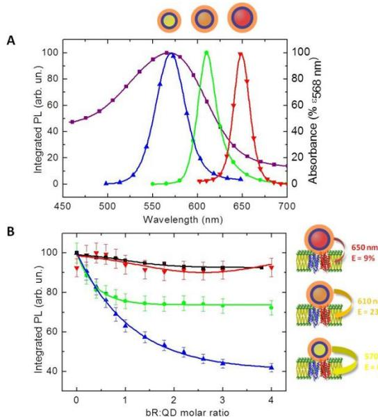
Figure 2. Experimental effect of variation of the overlap integral between QD fluorescence emission and bR absorption on the efficiency of energy transfer within self-assembled bR–QD hybrid materials.
