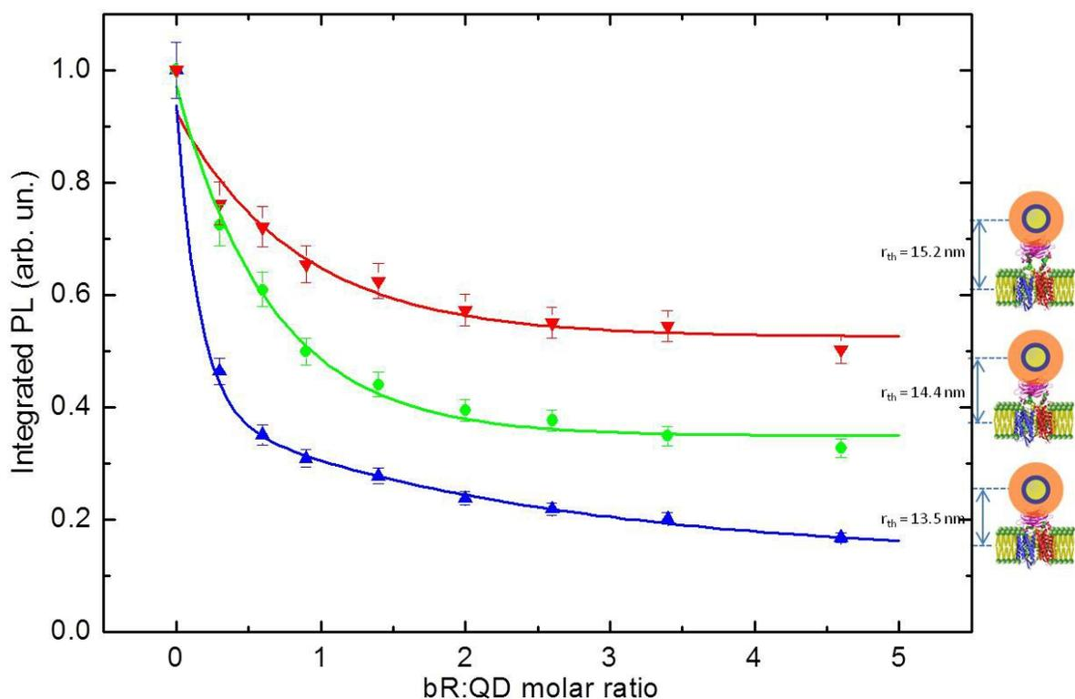
Figure 4. The efficiencies of energy transfer within QD–bR hybrid materials engineered through biotin–streptavidin linkage of streptavidinated QDs to PMs biotinylated using modified biotin linkers of different lengths.
