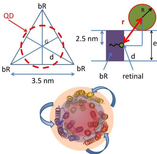
Figure 1. The multiple-acceptors FRET geometrical model based on the structural results of Refs. 20, 21 and illustrating the result of the use of Eq. 4 to calculate the theoretical donor–acceptor distances in the bR–QD nano–bio hybrid material.
