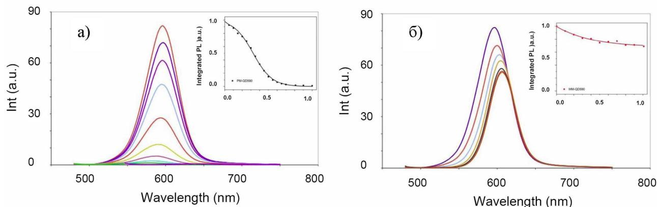
Figure 2. PL intensity as a function of the bacteriorhodopsin to quantum dot (QD) molar ratio. Variation of integrated PL of CdTe QD590 ( $\lambda_{em} = 590$  nm) as a function of the concentrations of (a) purple membranes or (b) white membranes. The concentration of QDs was fixed at 1.4  $\mu$ M. The optical densities in these experiments were always about 0.07–0.08.
