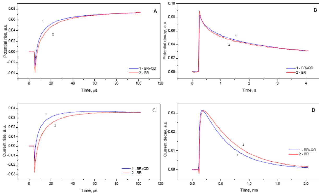
Figure 6. Kinetics of the (A, B) photopotential and (B, C) photocurrent generation in an oriented PM film containing QD570 (curves 1) and not containing quantum dots (curves 2 serving as control).
