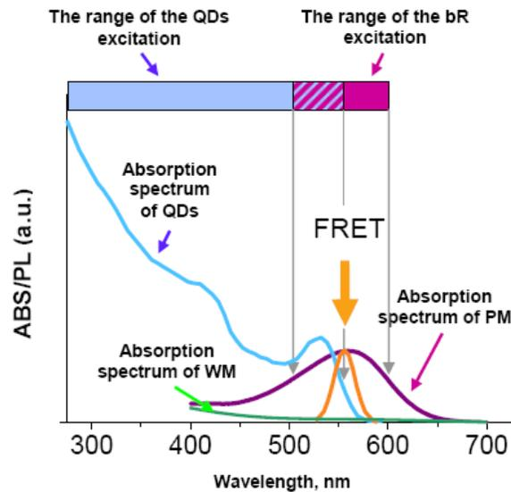
Figure 1. Optical properties of bacteriorhodopsin (bR) in purple and white membranes (PMs and WMs, respectively), and the scheme of energy transfer from quantum dots (QDs) to bR. The UV-vis spectra of PMs (the purple line), WMs (the green line), and one of the types of QDs used in the study (the blue line), as well as the PL emission spectrum of these QDs (the orange line), are shown. The spectral regions of the bR and QD effective excitation are shown as purple and blue bars, respectively.
