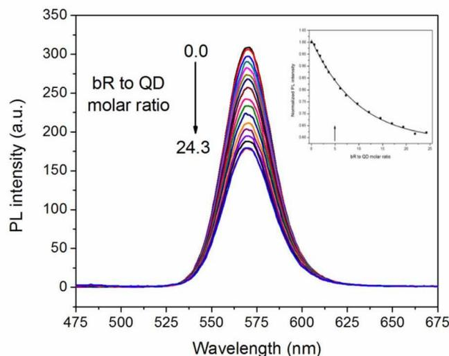
Figure 3. Initial QD concentration was  $\sim 0.9 \mu\text{M}$ . Excitation at 450 nm. The arrow indicates the bR to QD molar ratio used in photoinduced pH response measurements. A decrease in the QD PL of  $\sim 17\%$  was observed at this ratio, which agrees with the maximum increase in the proton pumping efficiency of 15% and FRET efficiency of 18% determined from time-resolved PL measurements (Table 2).
